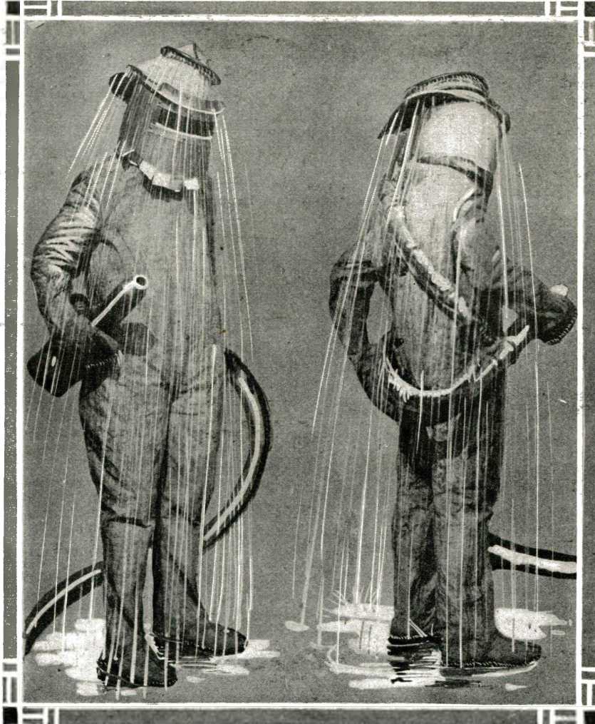
The Latest Thing in Firemen's Suits—It Sprays a Sheet of Water Down Between the Inner and Outer Coverings, as Well as Providing an Outer Water Curtain as Shown. This Water Curtain Protection is Supplied From the Main Fire Hose in the Manner Made Evident.
